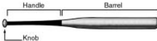
Figure 7.3 Parts of the bat.
